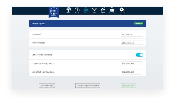
The **network port 2 is always in the LAN network**. The gateway address of the LAN network can be entered in the "IP Address" field.
