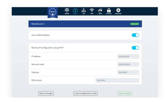
The **network port 1** by default si defined as WAN port and receives an IP address via DHCP. If required, this IP address can be defined statically. When used as a WAN port, the Internet traffic is sent via this interface, even if there is a mobile data connection.
