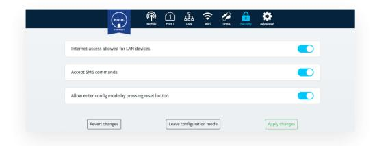
The setting "nternet-access allowed for LAN devices" allows you to allow connections from devices from the LAN network to the Internet.
