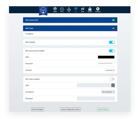
The WiFi can be used as an access point for the LAN network. The **password** corresponds to the **serial number** of the gateway and by default it is **switched off**.
